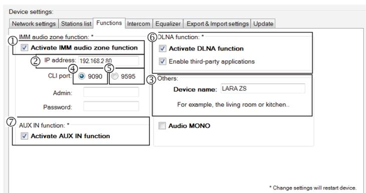
Function IMM Audio Zones: used for already installed iNELS system, where the LARA payer is a fully functional Audio Zone.
