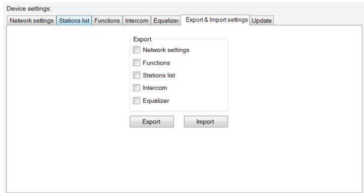
Export & Import settings: With these functions, you can easily back up and restore selected items - network settings, features, station list, intercom and equalizer. Created backups are in the \*.lcf format - backups of station lists from older firmware are not compatible with this system.
