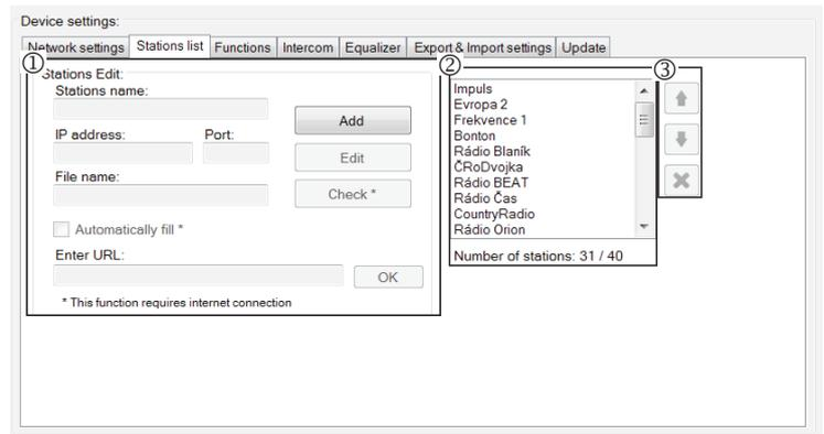
Adding new radio stations: after pressing the „add“ button, you begin entering the stream parameters into the relevant fields.
