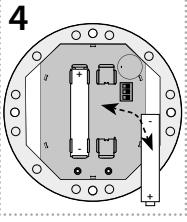
Insert / remove the battery into the detector according to the required function, ie: 1x battery insertion / removal - function 1, 2x battery insertion / removal - function 2... Each insertion must be signaled by flashing blue LEDs, there must be a delay of 1 s between individual inserts.
