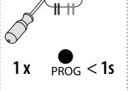
Press of programming button on receiver RF shorter then 1 second will finish programming mode.
