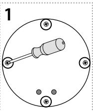
Use a screwdriver to open the detector.
